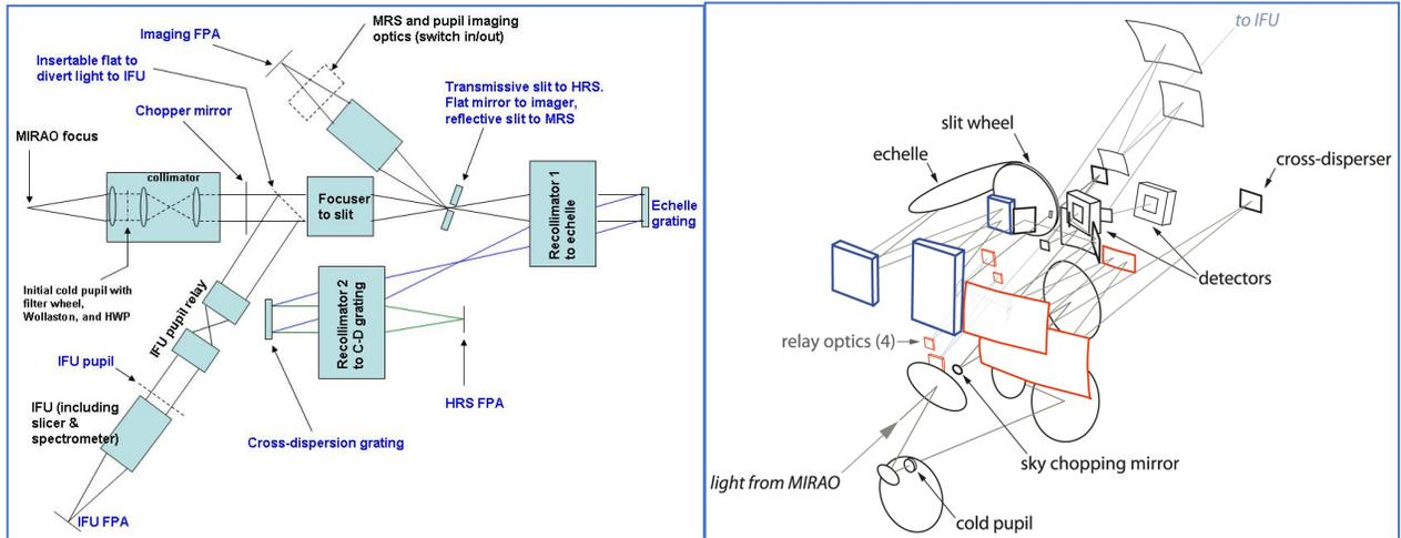
Figure 6. Feasibility-level MICHl design showing the integral modularity (left) and schematic design (right).
