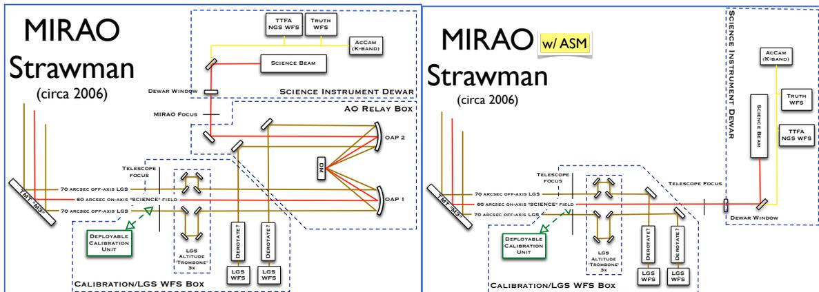
Figure 5. MIRA0 schematic design before ASM deployment (left) and after (right).
